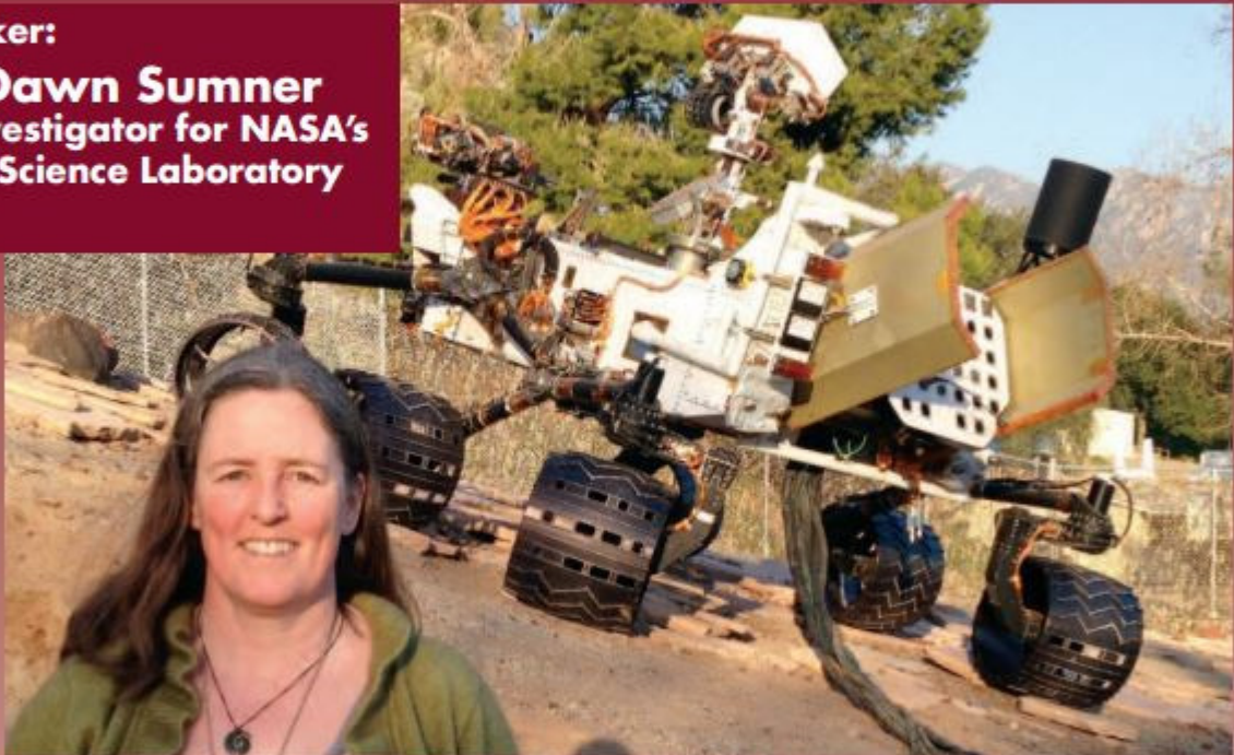
The rover in the background is Curiosity's twin at JPL, used to test commands before sending them to the real rover.
